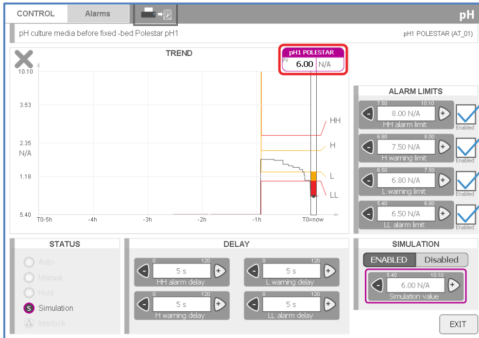
Figure 76: Warning and Alarm levels highlighted in pH auto-trend window
