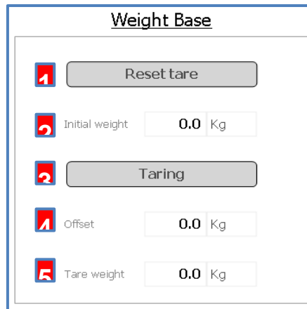
Figure 34: Weight base Calibration dialog box – 1) RESET TARE button, 2) Initial weight = raw data without Tare offset, 3) TARING button, 4) Currently applied Offset, 5) Live weight with Tare offset applied.
