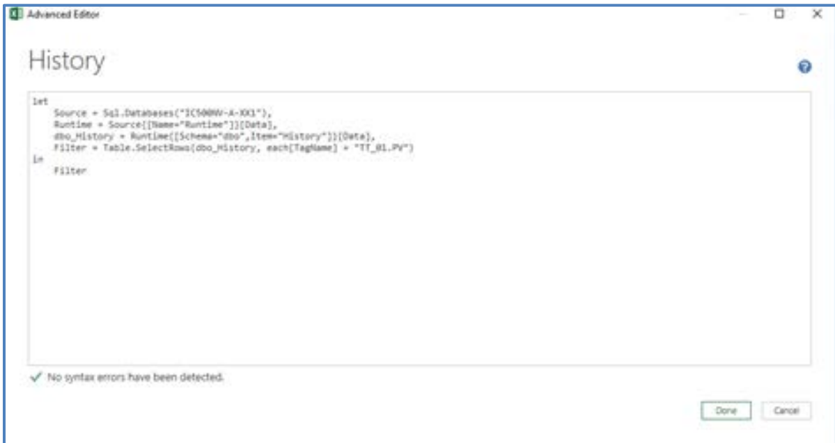
Figure 139: E.g. Query to get the data for TT_01 Tag (temperature of the bioreactor)
