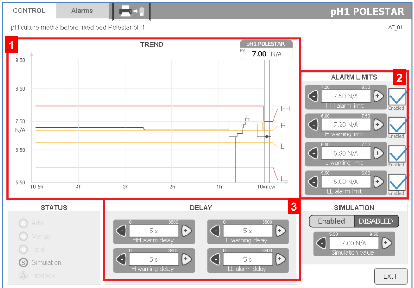
Figure 12: Sensor configuration box – 1) Sensor measure trend over last 5 hours, 2) Alarm limits set-point boxes and Enabled checkboxes, 3) Alarms delay set-points.
