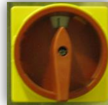
Figure 4-2: Main Power Disconnect Switch
