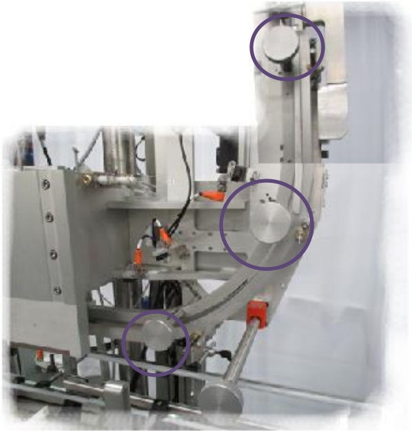
Figure 5-20: Installation of the chute—Silver Knurled Knobs
