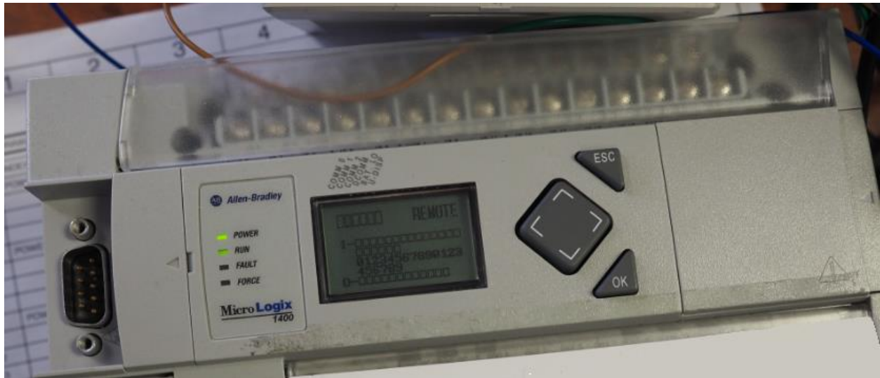
Figure 9-1: Normal PLC with batteries at full capacity
