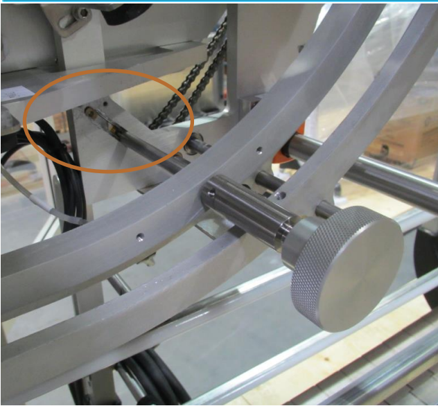
Figure 5-22: Proper positioning of the chute
