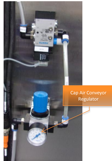
Figure 5-40: Cap Conveyor and Elevator Regulators
