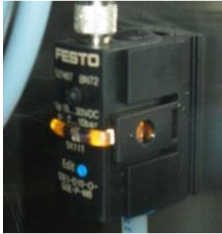
Figure 5-41: Low Air Pressure Switch
