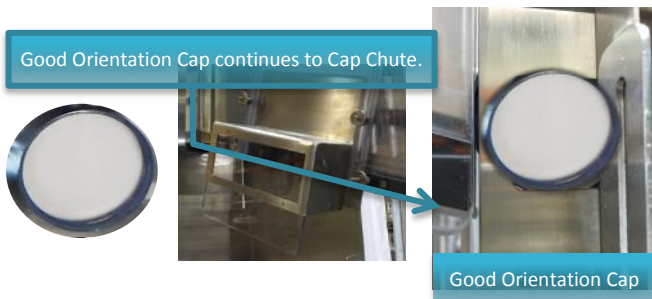
Figure 5-13: Cap Side Selection #2 (Good Orientation Cap Goes to Cap Chute)
