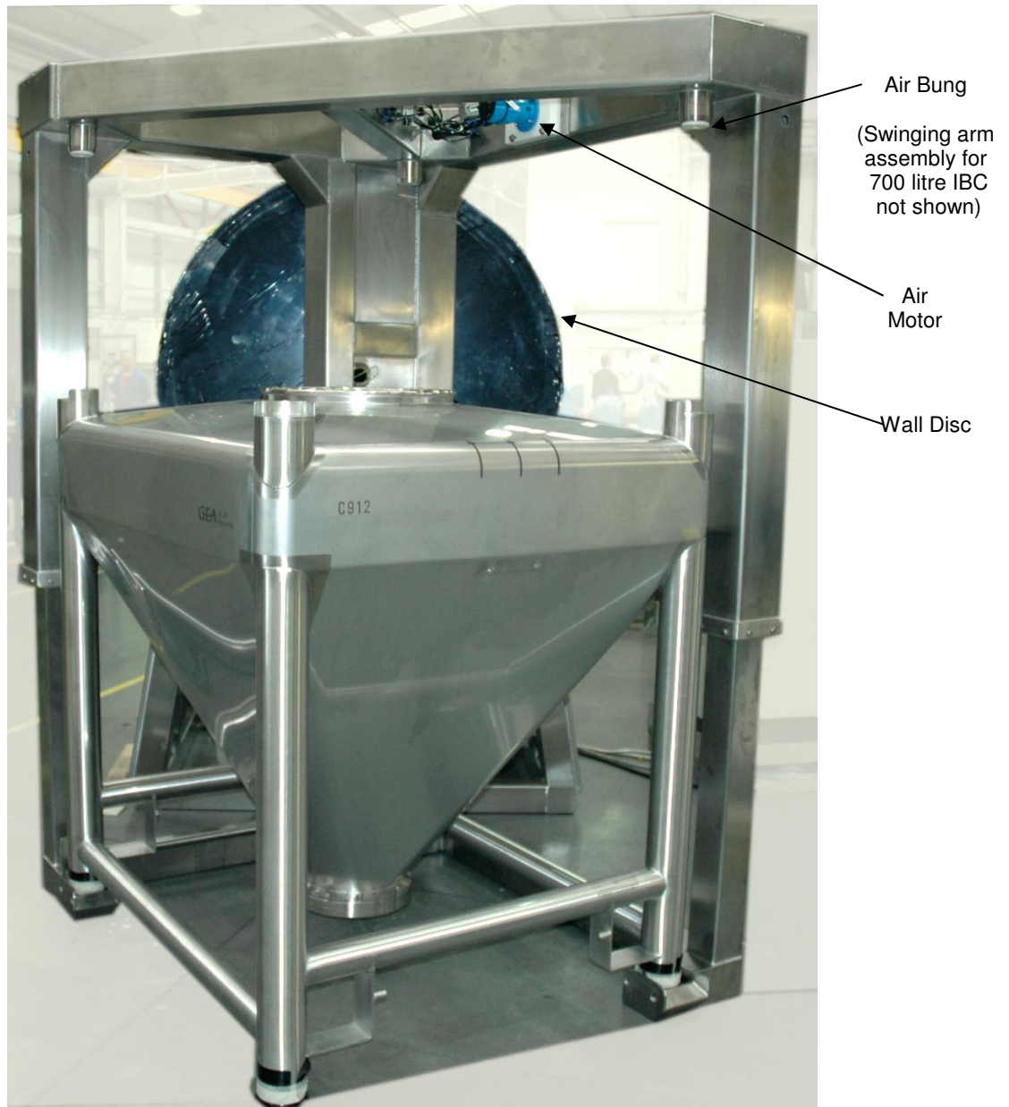
Fig 8 - Blender – Cage Assembly with IBC in position
