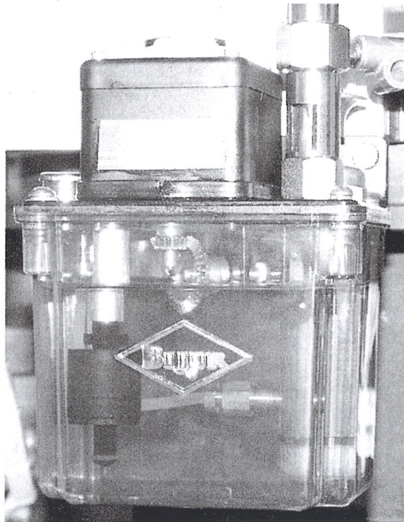
Figure 28 – The photo shows the oil pump.
