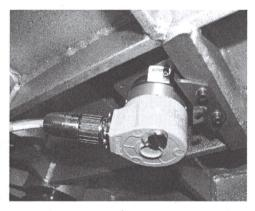
If the encoder malfunctions, the control system stops the machine and displays a message on the monitor.
