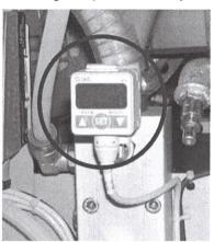
When the pressure is below the minimum set value, the control system stops the machine and a message is displayed on the monitor. A pressure value too low (under the lower limit set) compromise the right machine functioning.
