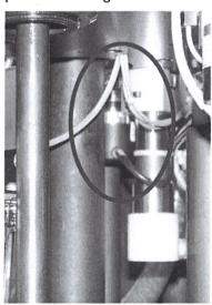
If the encoder malfunctions, the control system stops the machine and displays a message on the monitor. Each dosing unit is equipped with a chamber encoder for the adjustment of relevant dosing chamber.
