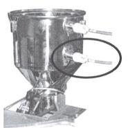
The system enables the automatic loading device when capsule level falls to the set minimum level detected by the sensor.
