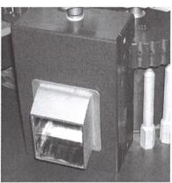
This enables the system to check whether any non-conforming capsules have been rejected by the previous devices. If a non-conforming capsule is detected during the production outfeed stage, the system stops the machine and a message is displayed on the monitor.
