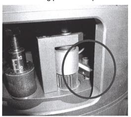
This sensor is triggered when the minimum compression limit is reached. During compression adjustment, if the sensor is triggered before the adjustment is completed, the adjustment command is aborted and an alarm message is displayed within the drive control function (on the panel). Moreover, it is possible to check the alignment between the value displayed on the panel and the real mechanical value if the sensor intervenes within 1 mm of the minimum value.
