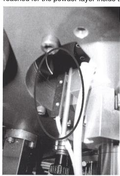
When the powder layer reaches the maximum level the control system stops the machine and displays a message on the monitor.
