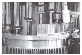
This sensor detects the drop in the powder level and sends a signal to the system indicating the need to restore a sufficient powder level inside the rotary container.
