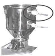
The system stops the automatic loading device when capsule level reaches the set maximum level.
