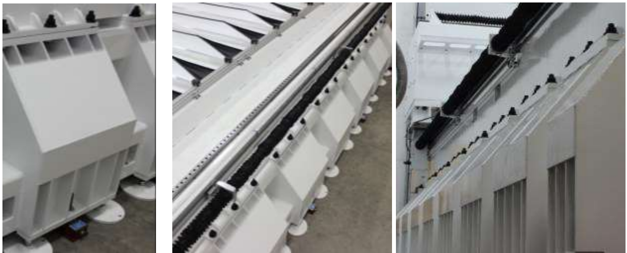
Shown – Y and V Upright Design – Single 45mm Rail with Roller Bearings on Y and V.
