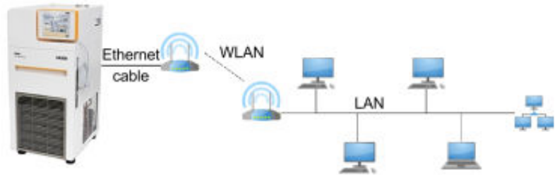
Fig. 16: Connected via LAN and WLAN
