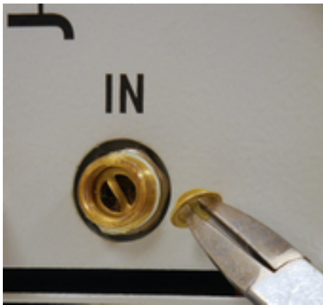
Fig. 74: Dirt trap installed, with pliers
