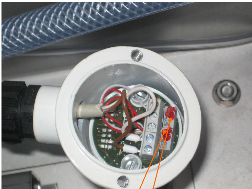
PT100 sensor with built-in converter ( at the top )
