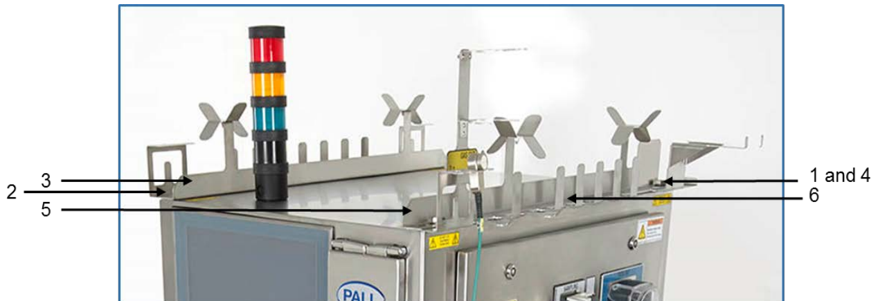
Figure 11: Assembly position of tubing holders items on iCELLis 500+ control system (the item number corresponds to Table 4)
