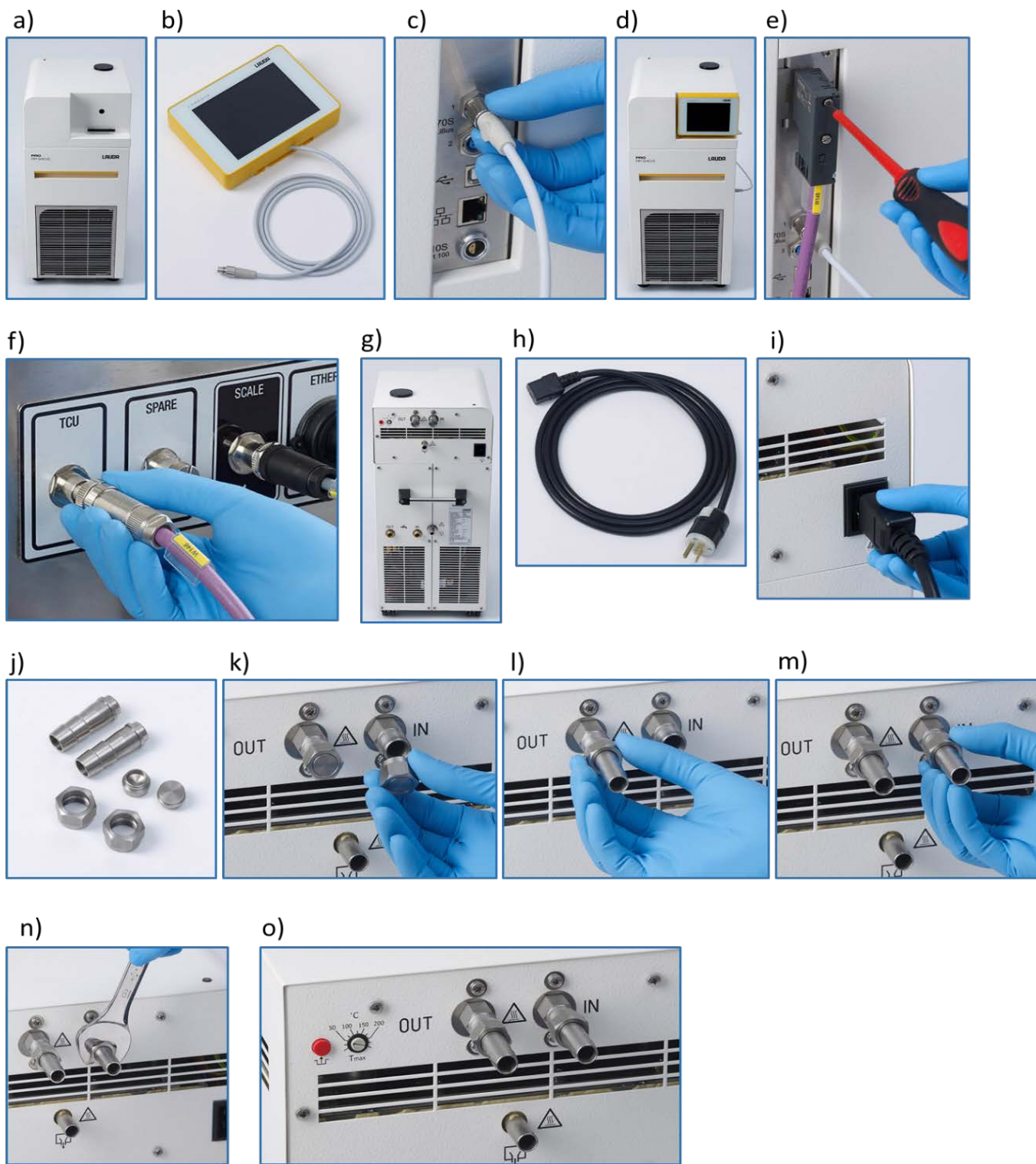
Figure 26: TCU installation procedure – a) TCU out of the box, b) Command touch panel, c) Connection of touch panel cable, d) TCU with Command touch panel, e) Connection of Profibus connector on TCU, f) Other end of Profibus cable on iCELLis 500+ bioreactor, g) TCU rear side image, h) Power cable, i) Connecting power on rear side of TCU, j) Barbed connectors for IN/OUT line on back of TCU and closure nuts, k) Removing existing closed nuts, l,m,n,o) fixing the connectors with nuts on IN/OUT lines.
