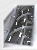
**Bi-directional Scraper System:** Blentech patented scrapers cover the total heat transfer surface area, and are designed to maximize heat transfer and minimize/eliminate product build up.
