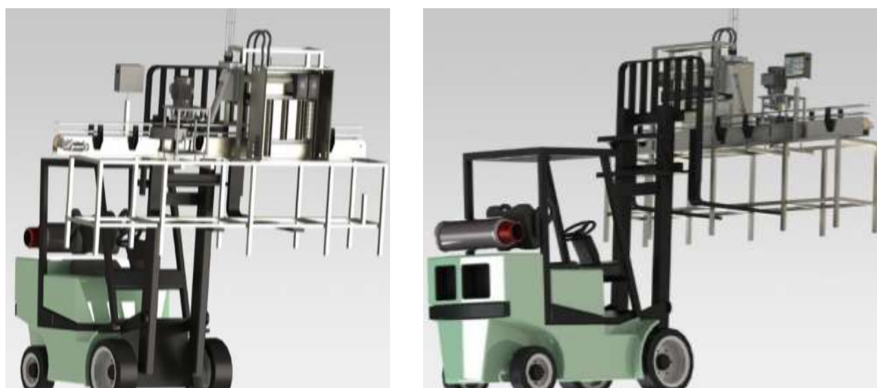
Figure 5 Forklift moving Cask ACS into position
