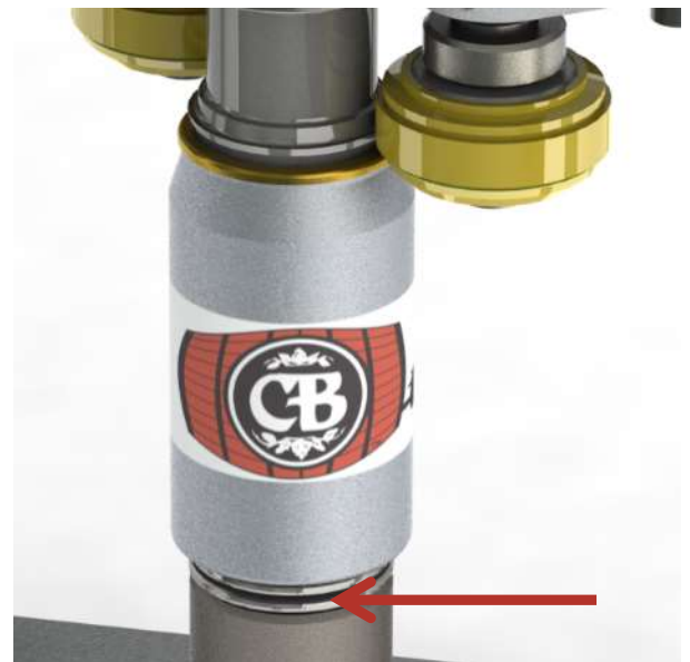
Figure 42 Can Table Height Adjustment
