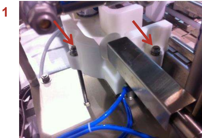
Figure 29 Adjusting height of the slide table
