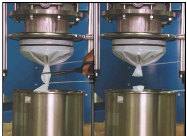
Fig. 18 Cutting apart/separating the dust bag
