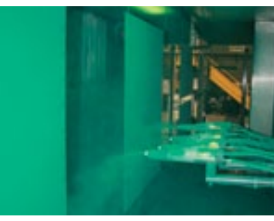
Individually Powder Coated Farr Gold Series components are individually powder coated prior to assembly for superior corrosion resistance.
