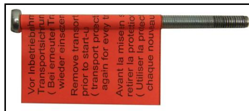
Fig. 95. Transport securing of the web-edge control unit
