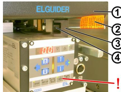
Fig. 94. Transport securing of the web-edge control unit by means of cylinder head screws M4x70 with red flag
