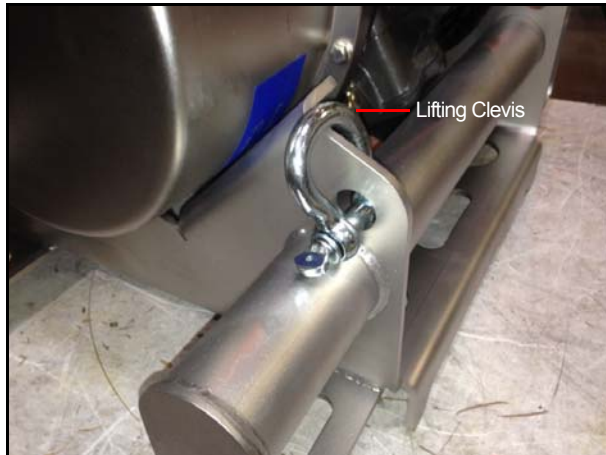
Figure 8-4 Drive Installation Tool with Clevis at Lifting Point
