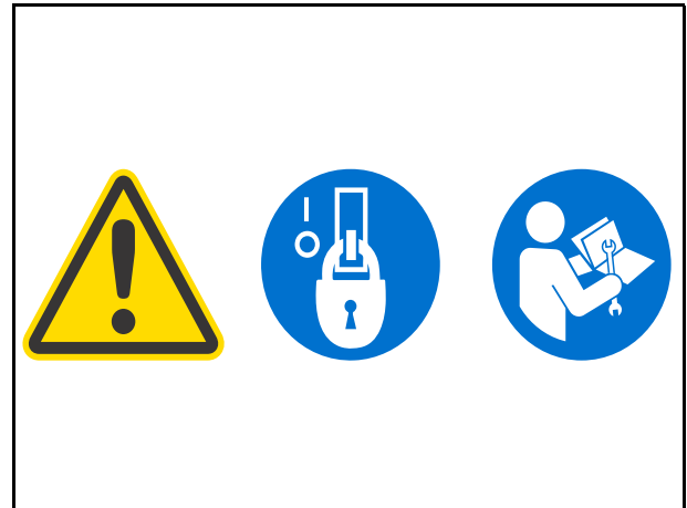
Figure 1-1 Affixed to the Iso-Flo Shaker: Warning, Lock out in De-energized State. Refer to Technical Manual for Service
