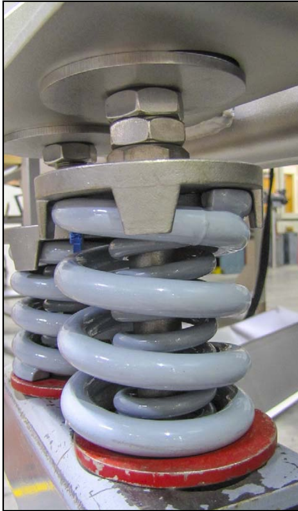
Figure 3-6 Coil Isolation Spring-AWC Floor Mount
