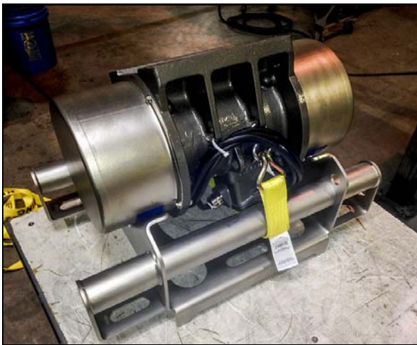
Figure 8-2 Drive Installation Tool with Drive Attached
