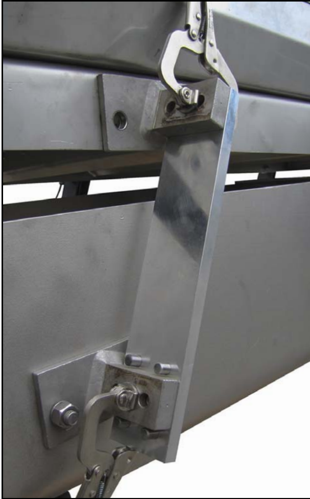
Figure 5-30 Arm Transfer Jig for Marking Arm Hole Locations -To Realign Beds With Bolt-on Arm Brackets, Key P/N 1077800
