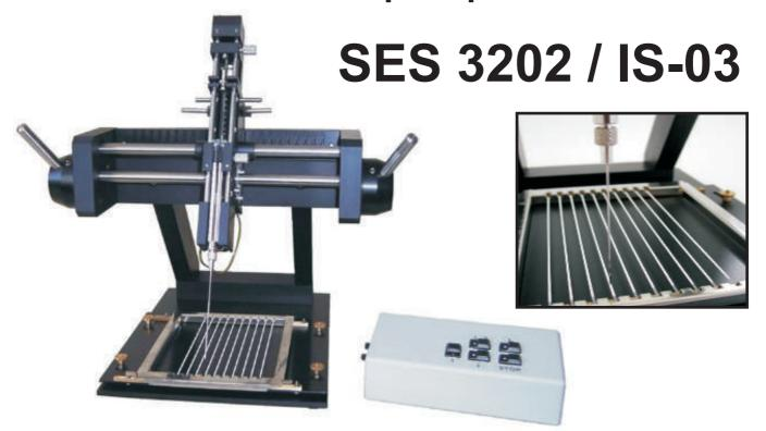
SES Model 3202 Autospotter for TLC/FID techniques is a new precision instrument specially developed for applying sample solution onto the sintered silica gel surface of a Chromarod. The smaller and more concentrated the sample spot, the better the resolution obtained after development of the Chromarod in a TLC chamber (3201).
