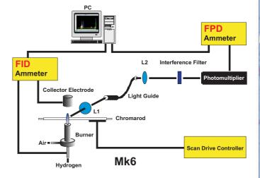
The TLC/FID Analytical System IATROSCAN MK-6(s) was developed for the Analyzing of organic Substances, which show no UV- Absorption and no Fluorescence, and give difficulties by analyzing with GC.
