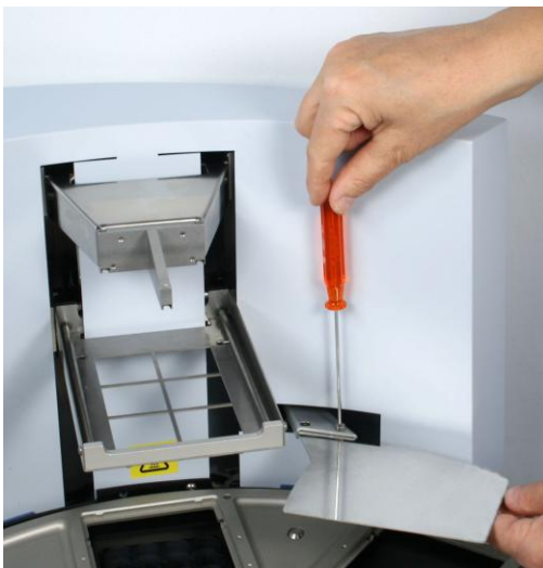
Figure 10. Fastening / loosening the shield plate (A) and when in place (B)
