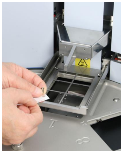
Figure 6. Removing the transport lock of the heating block (B)
