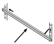
Suspend the rails at the desired height, by inserting into the rear clip-in strip first and then clipping in at the front.
