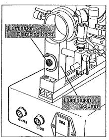
①When shipped from the factory, the illuminator clamping knob is fastened to the illumination column. To install the illuminator, tum the illuminator clamping knob counterclockwise to remove it.
