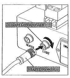
③Put the light connector, with its slotted part facing upward, into the light connector jack marked "LIGHT" on the back panel. While carefully pressing the cover of the light connector, turn it clockwise to lock it firmly.
