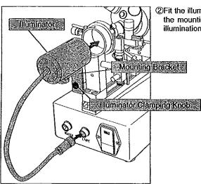
②Fit the illuminator clamping knob (removed in ①) into the hole in the mounting bracket and fasten the illuminator securely to the illumination column.
