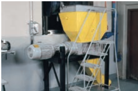
4-SHRED-H with Custom Hopper and Discharge Chute
