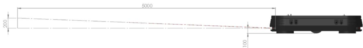
Figure 2 OTTO 1500 V1.2 SDV Open Detection Range (mm)
