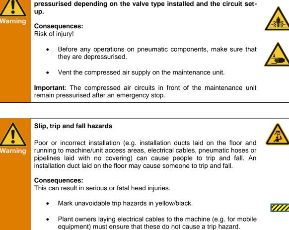
When installing the required installations (ducts, lines, cables, hoses and pipes), qualified staff must ensure that these do not cause a trip hazard.
