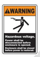
Hazardous voltage or presence of voltage which could cause serious injury are highlighted by signage on the instrument
