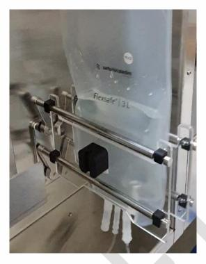
The paddle mixer speed is controlled on the faceplate by a '% speed' control. The table below shows the conversion between '% speed' and number of oscillations per minute, where a single oscillation is the paddles moving from open, to closed, to open again.
