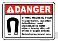
Take care when interacting with the MSP as the magnetic platen uses a strong permanent magnetic field. Can be harmful to pacemaker wearers and others with medical implants. Keep tools and other metal objects away.
