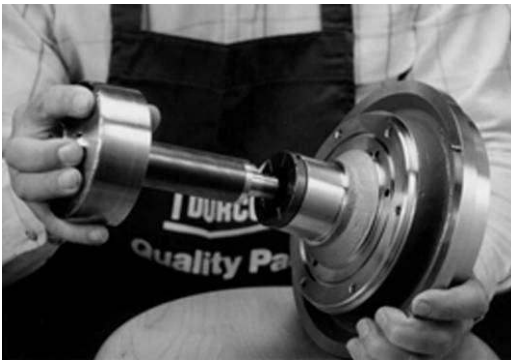
Figure 6-36 Inner magnet/shaft assembly installation
