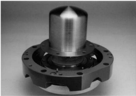
Figure 6-8: Containment shell removal
