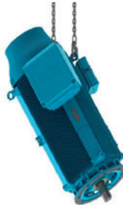
Figure 4.14 - Lifting HGF and W50 motors by the eyebolts at the non-drive end
