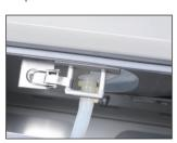
Bottom outlet port securely clamped and clamps locked into place ensuring no possible lateral or up and down movement of the portbiocontainer joint
