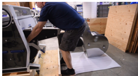
11. Slide fan housing off pegs and remove from the body. Place it on the foam sheet with the separator.
