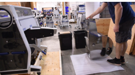
10. Place hand in the gap to support the weight of the separator and pull it the rest of the way out. Place separator on foam sheet
