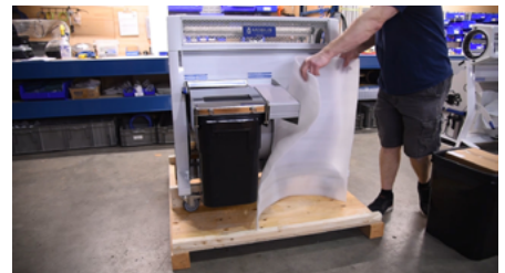
6. Place foam sheet on ground to be used as a protective barrier for other removed components
