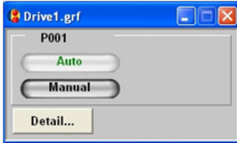
Pump Control Mode Pop-Up – Pump Currently in Auto
