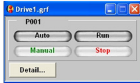
Pump Control Mode Pop-Up – Pump Currently in Manual
