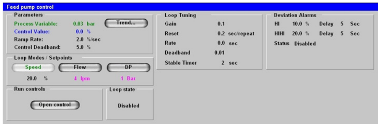
Feed Pump Control Status Display with the Detail screen open
