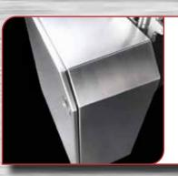
• All *i*-Cabinet surfaces and virtually all other areas inside and outside the machine are designed with a 3-5 degree slope to aid in runoff and keep the machine cleaner.
