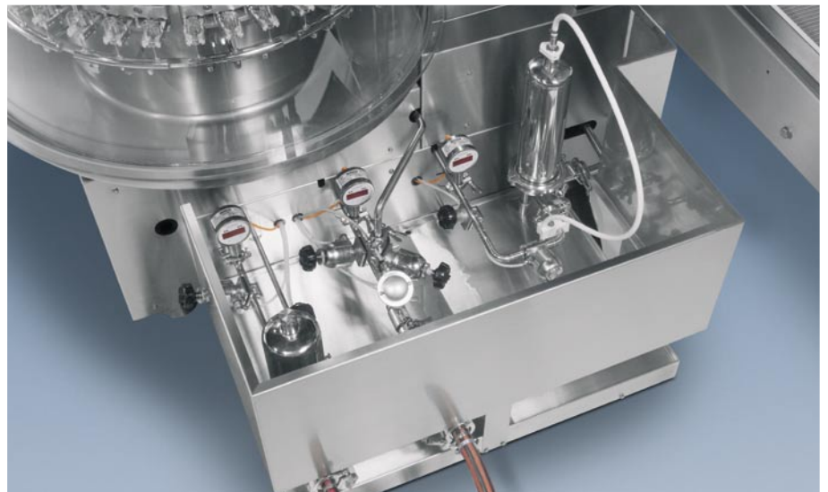
Filter plate with short pipes
