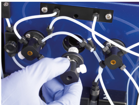
Figure 7.13: Detach the valve.
