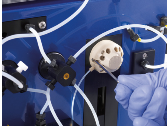
Figure 7.17: Unscrewing the dilutor valve's socket screws.
