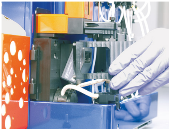
Figure 7.21: Dismantle the washing station.
