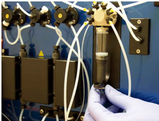
Figure 7.6: Place the plunger in its fitting and tighten the plunger lock screw
