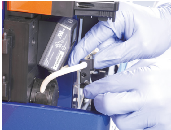
Figure 7.22: Removal of the waste distributor.
