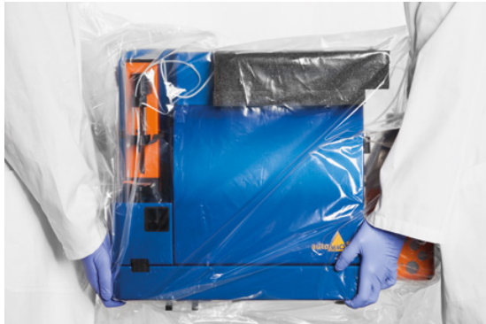
Figure 2.4: Two people are required to lift the autoMACS Pro.
