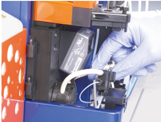
Figure 7.23: The draining tube is attached.
