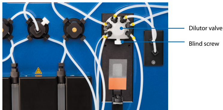
Figure 3.3: Fasten the syringe at the dilutor valve.
