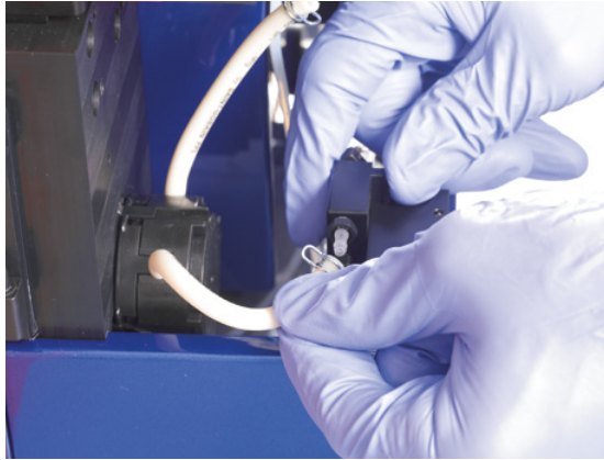
Figure 7.24: Disconnecting the tubing from the waste distributor.
