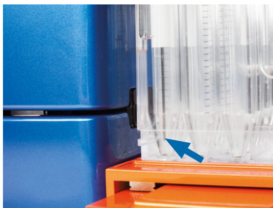
Figure 5.7: Test position: Uptake needle position in the Chill Rack.
