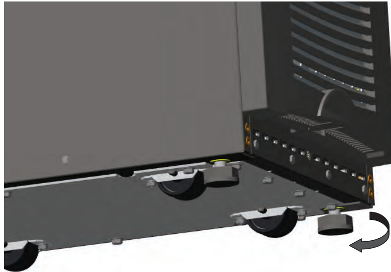
Figure 34. Lowering the Leveling Feet
