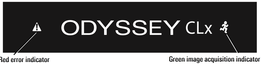
Figure 4-2. Location of the green image acquisition light and red error light.
