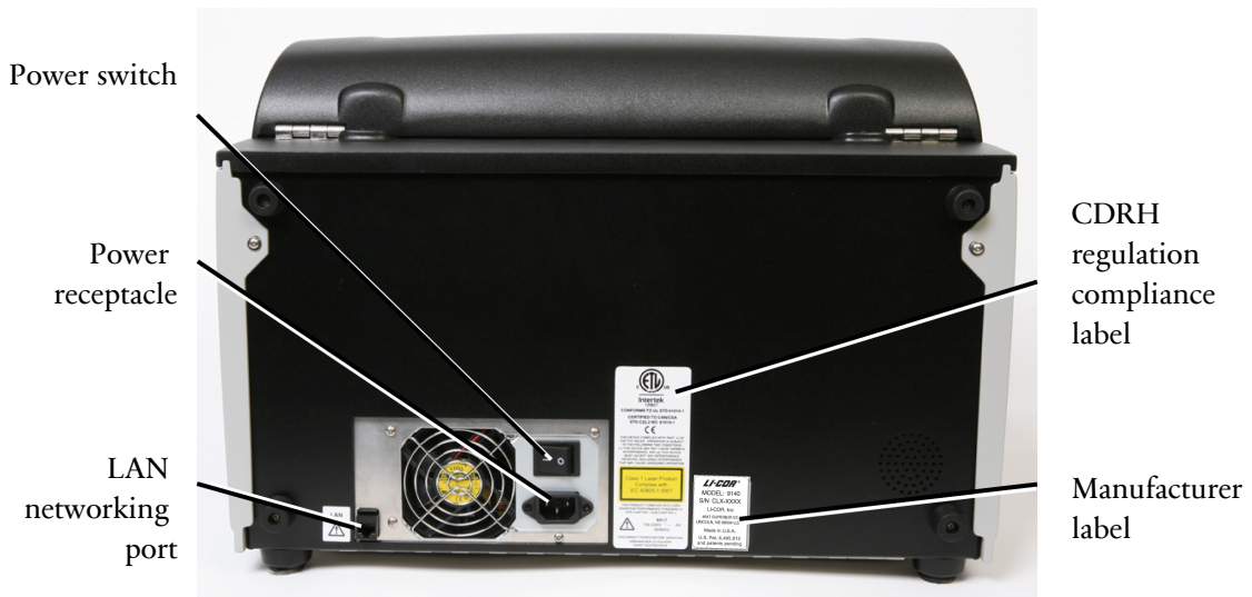
Figure 4-3. Closeup of the Odyssey® CLx Imager rear panel showing the power receptacle and LAN port (use only the supplied networking cable). Also shown are the CDRH regulation compliance label, the manufacturer label and the power switch. The power switch should be left in the 'on' position. Note: The appearance of your instrument's back panel may vary slightly from the one shown.
