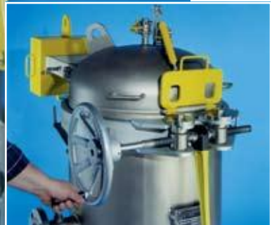
HANDWHEEL OPERATION OF TURNBUCKLE MECHANISM
